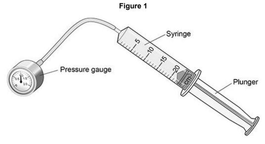
When the plunger was pushed slowly into the syringe, the temperature of the air stayed the same.
