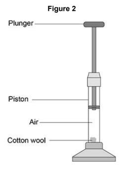
The plunger is pushed quickly downwards and compresses the air.
